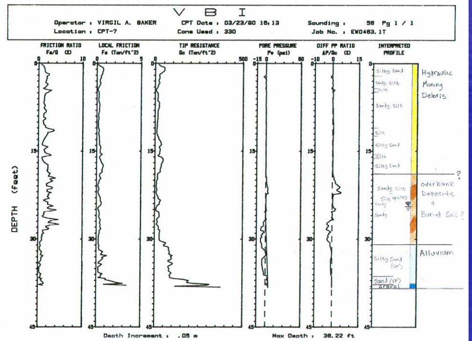
**CPT logs can be very useful for analyzing *discrete horizons*, *zones of saturation*, and unraveling subsurface stratigraphy; to ascertain the *continuity* of various units.**
