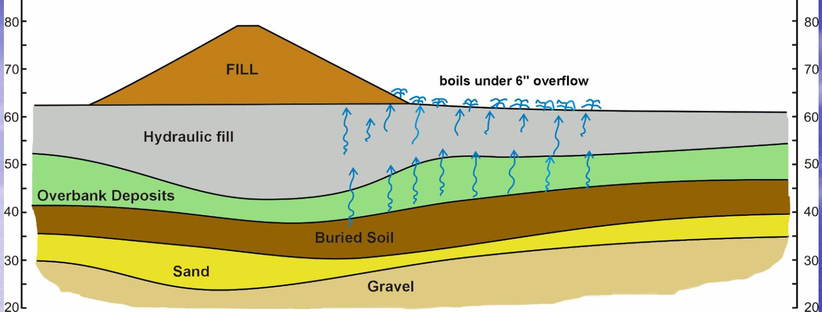
**Hydraulic uplift from confined gravel aquifer under considerable pressure head. As head increases, unconsolidated low density materials turn to soften and lose strength, turning to 'mush'**
