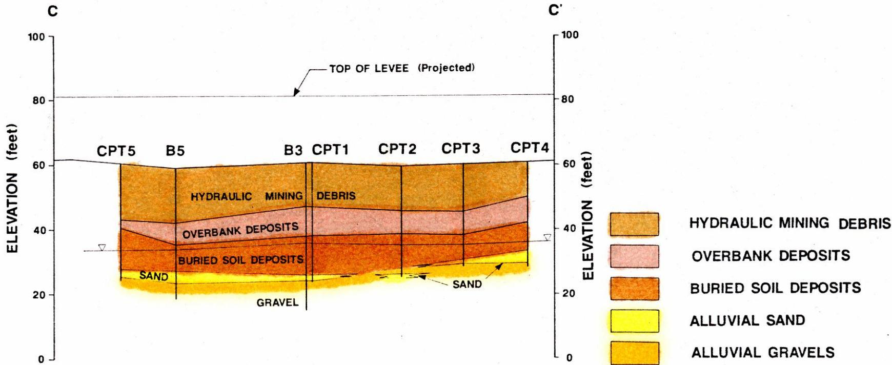
**The underlying units appear as rather ordinary layers in this section, parallel to the axis of the failed levee.**
