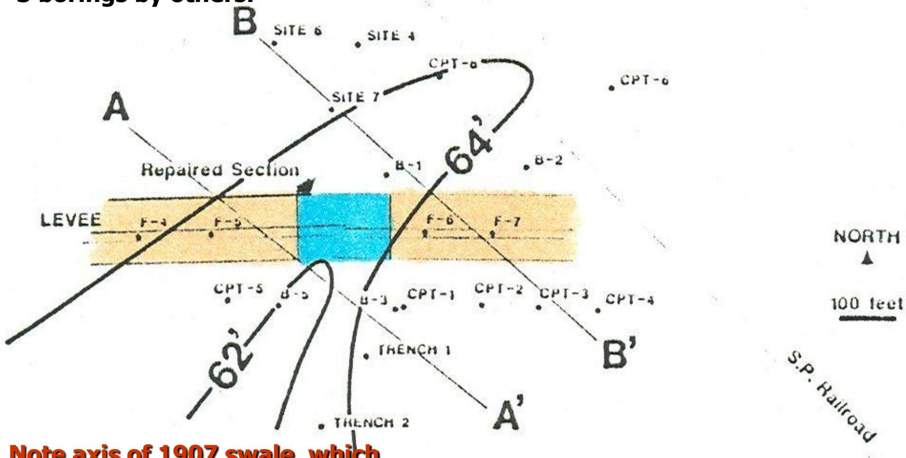
Note axis of 1907 swale, which coincides with the 1986 breach
