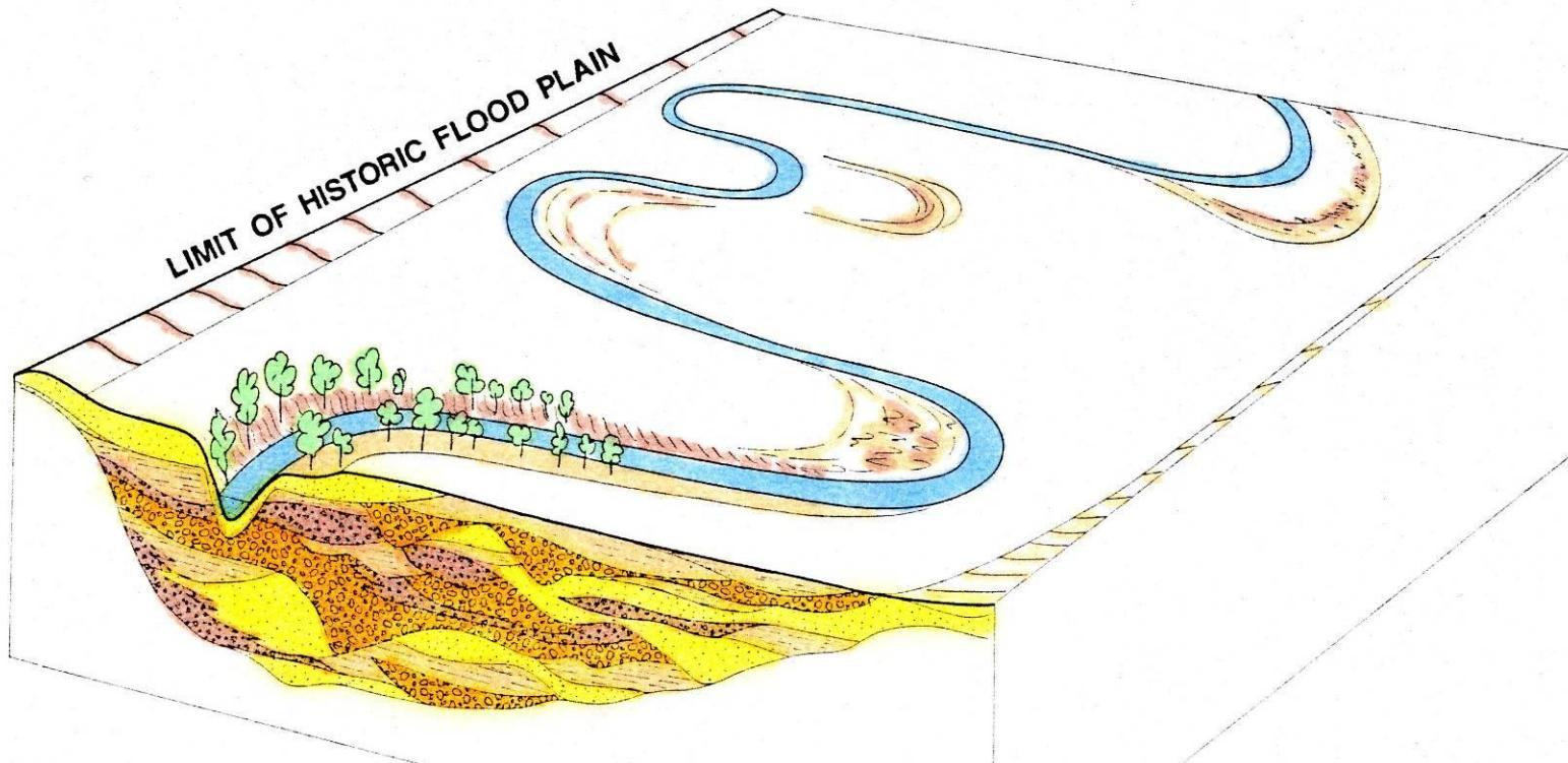
The  $D_{15}$  particle size tends to control permeability; and  $k$  can vary by four orders of magnitude in adjacent channel deposits. If you miss the high permeability channels, you fail to characterize the site conditions for any meaningful seepage analyses.
