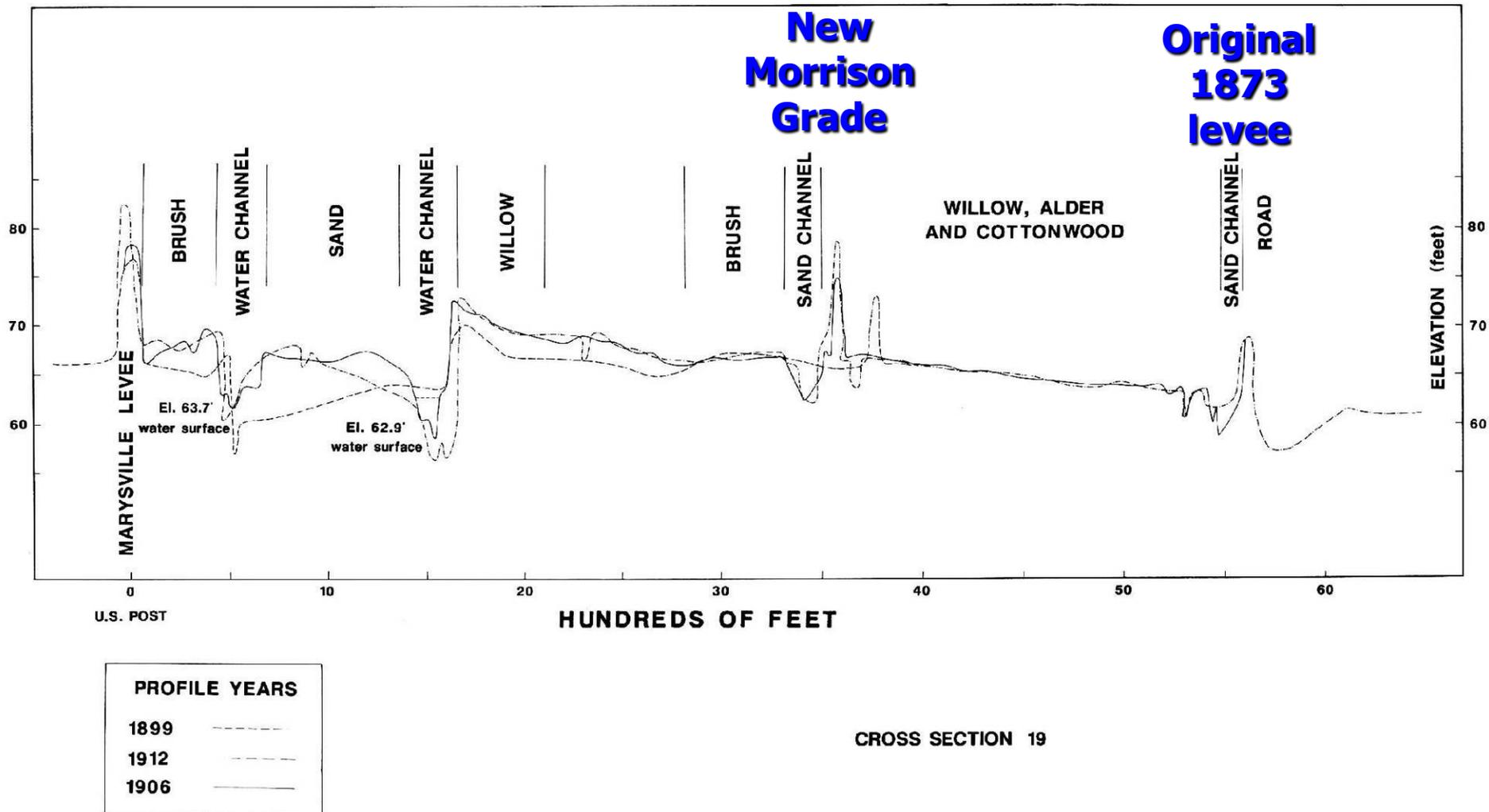
● Cross section of the lower Yuba River prepared by the California Debris Commission in 1907. Note gradient of the clogged flood plain, diminishing with increasing distance from the main channel.
