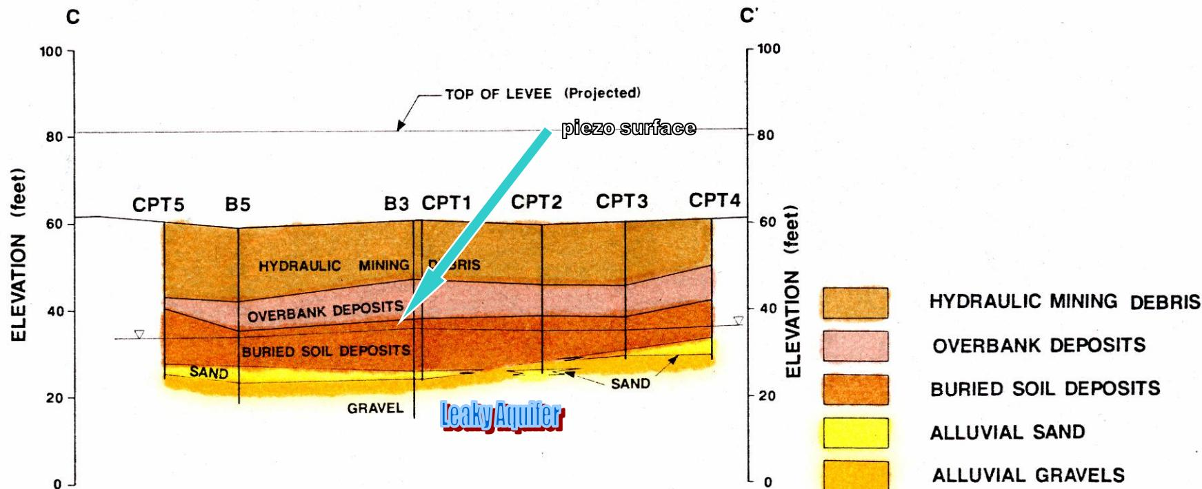
Pore pressures emanating from the cobble gravels extend into the low permeability paleosol cap. As soon as flood waters filled the Speckert gravel pit, that pressure head would have acted on the leaky aquifer, engendering considerable uplift
