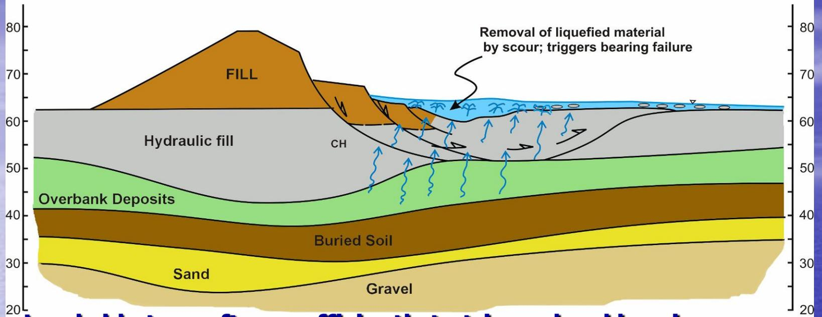
**Land side toe softens sufficiently to trigger local bearing capacity failure; which triggers retrogressive slumping, as lateral restraint is removed. This explains eye witness accounts.**
