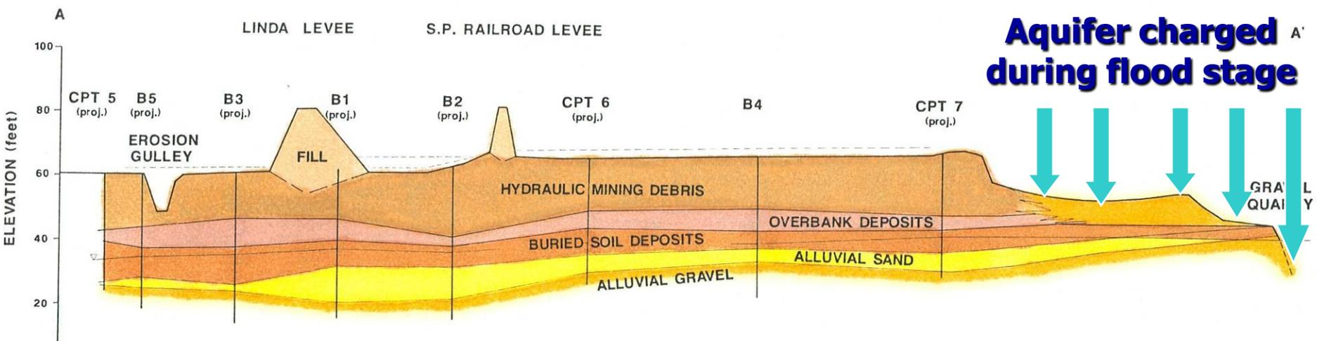
**Note upward dip of the alluvial gravels, into the gravel quarry**
