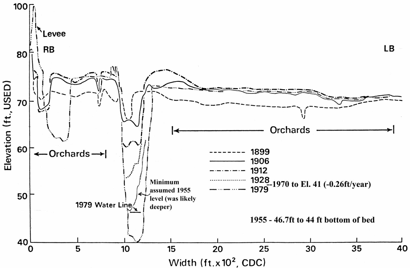
**By 1983, the main stem channel of the Yuba River retrenched itself to its pre-1862 level, as shown here. Orchards were planted on the mine slickens (silt).**
