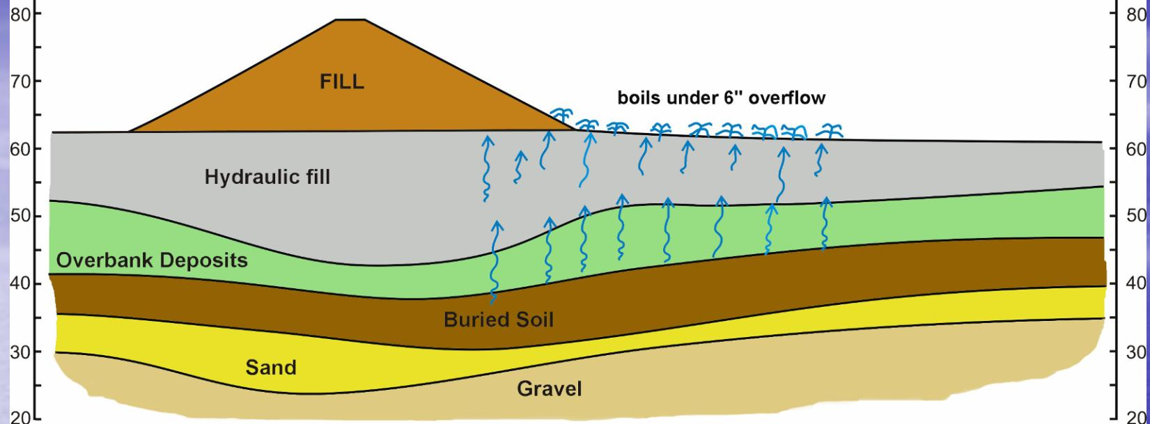
**Hydraulic uplift from confined gravel aquifer under considerable pressure head. As head increases, unconsolidated low density materials turn to soften and lose strength, turning to 'mush'**
