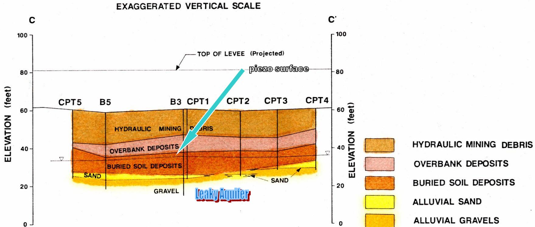
**Pore pressures emanating from the cobble gravels extend into the low permeability paleosol cap. As soon as flood waters filled the Speckert gravel pit, that pressure head would have acted on the leaky aquifer, engendering considerable uplift**
