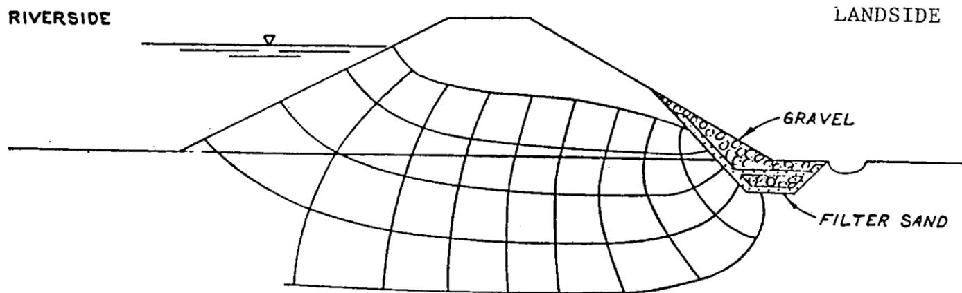
c. Pervious toe combined with partially penetrating toe trench
