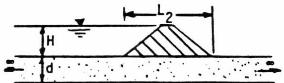
b. CASE 2 - Impervious topstratum both riverside and landside
